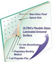
ULTRA is A D Metro's line of durable resistive touchscreen sensors. Our patented thin-glass lamination process provides a flexible pressure activated membrane forming a Glass/Film/Glass (GFG) resistive touchscreen solution that offers un-paralleled performance characteristics. A solution that combines the operational advantages of a resistive sensor with the durability of a glass surface.
