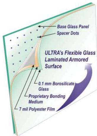
ULTRA is A D Metro's line of durable resistive touchscreen sensors. Our patented thin-glass lamination process provides a flexible pressure activated membrane forming a Glass/Film/Glass (GFG) resistive touchscreen solution that offers un-paralleled performance characteristics. A solution that combines the operational advantages of a resistive sensor with the durability of a glass surface.
