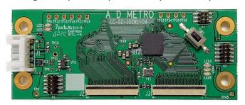
drivers making it compatible with any operating system that can operate with a mouse. It simplifies inventory for customers wishing to implement PCAP in their product offering but to only need one controller that can handle all their sensor size requirements. This is especially useful for field servicing as the customer
